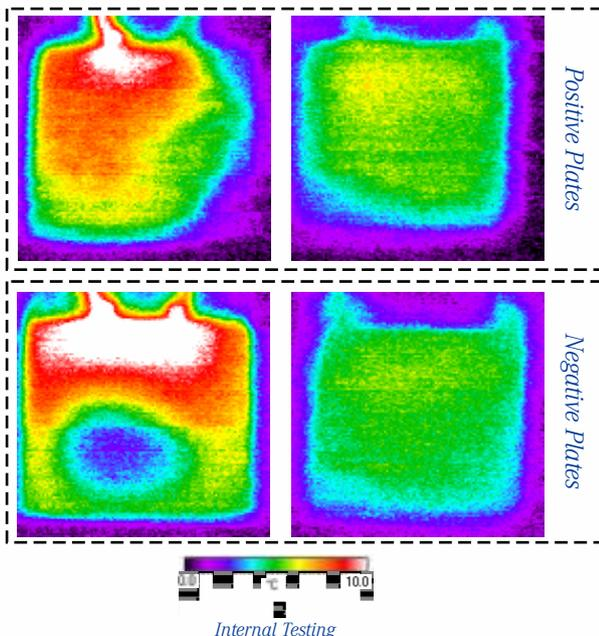
Infrared thermal images snapped at the end of a 5C (12 minute) discharge of both a Firefly 3D cell and a Traditional cell.
